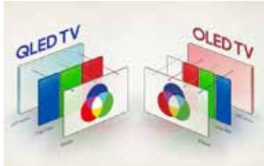
**Quantum-dot Light Emitting Diode**, is Samsung's answer to where the living room TV is headed. It uses 'quantum dots' which are tiny particles only a few nanometres in size, these particles are capable of giving off incredibly bright, vibrant,
